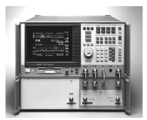
The Agilent Technologies 8542E EMI test receiver is designed for conformance testing to industry standards such as CISPR, EN, FCC, VCCI, and VDE.
